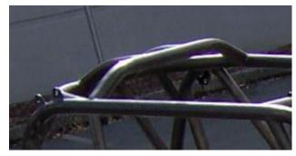
**6.4.7** Optional (Morris) "T" Bar may be included to top roll cage opening, ONLY after roll cage opening meets all other specifications as above. A minimum measurement of 380-mm (15") is required between the "T" bar rail and the front roll cage member. Main bars to be min. 1 3/8" x 095".
